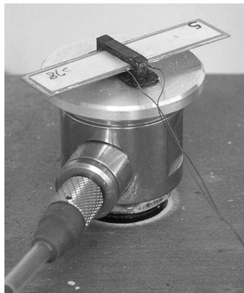
Fig. 3 The SLDMA mounted on an aluminum plate that is screwed rigidly into a force transducer
